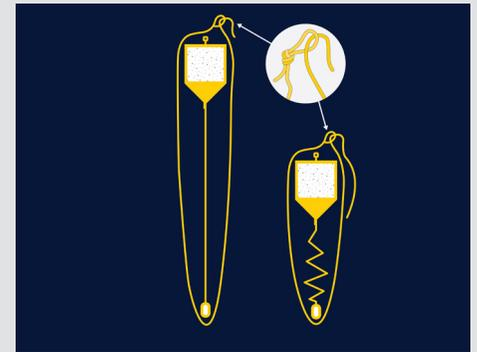
Aer-Flo can build a tapered barrier, or we can add furling lines so that the installer can drop the bottom of the barrier to a custom depth.
