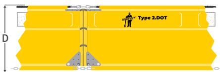
This is the workhorse of the TOUGH GUY® barrier line. Comes supplied with a top load cable and special stress plates for reinforcing the corners and is designed to handle more severe conditions. It is recommended for lakes, streams, inter-coastal and tidal areas where current velocities up to five feet per second are expected.
