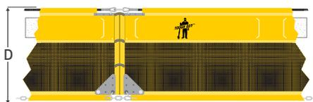
This is a special adaptation of the Type 2 barrier. Approximately 20% or more of the area of the barrier skirt fabric is replaced with a polypropylene filter fabric conforming to some State DOT specifications. The filter fabric is inserted to reduce the pressure on the curtain while retaining silt.
